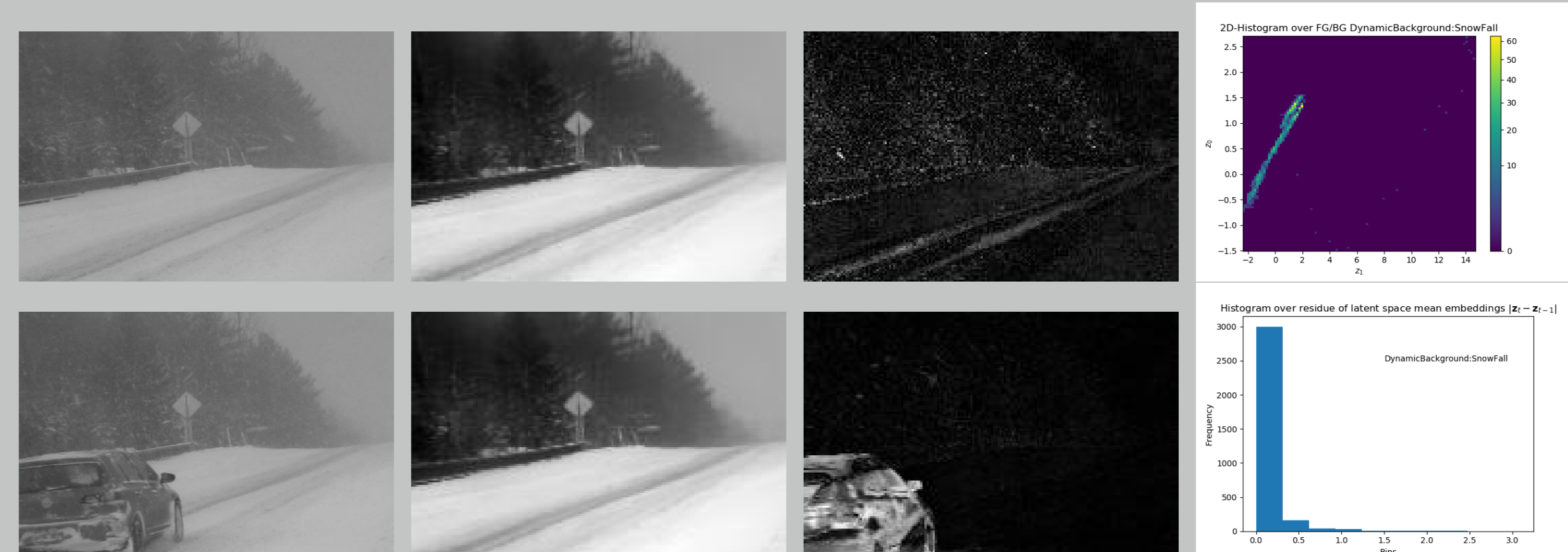
Figure 5: The input-output pairs and absolute value of residue between input-output pairs from a Convolutional VAE : top half without foreground bottom half with foreground. We remark that the dynamic background such as the snow has been removed. The right column demonstrates the 2d-Histogram over the latent space z of the CVAE (top) and the histogram over the temporal residue over z for the same test sequence.
